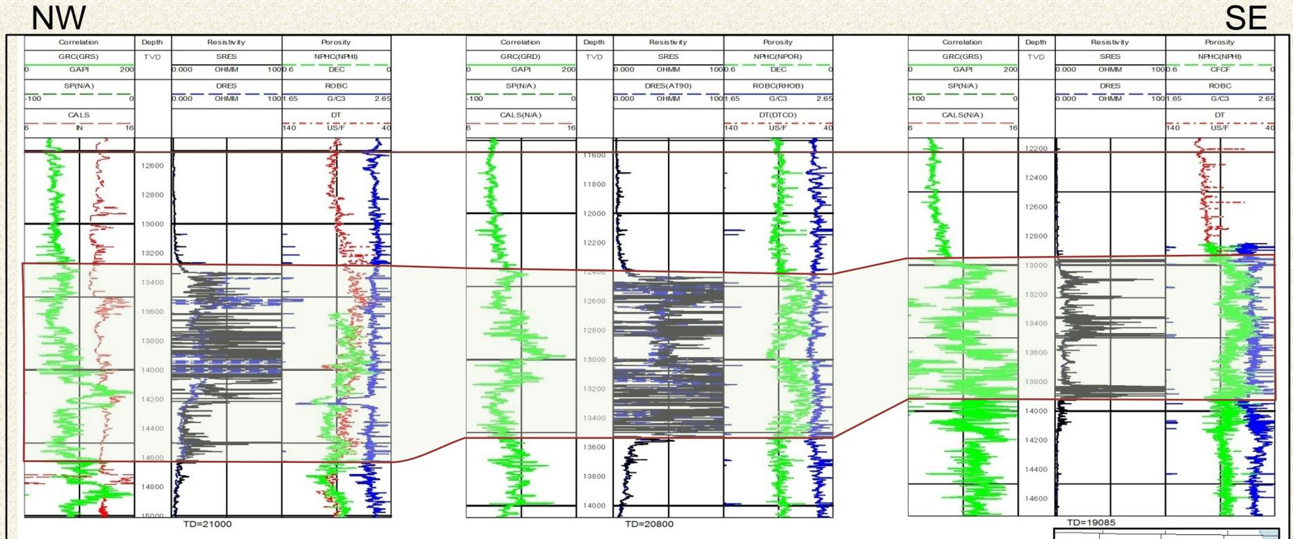
This high-resistivity Monterey facies is well developed on the deep eastern flank of the Lost Hills anticline. The facies begins to lose some of its distinctive resistivity character eastward onto the eastern platform of the Buttonwillow basin, although it maintains most of its thickness.
