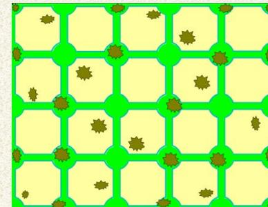
Mature Kerogen in Matrix With Oil in Open Pore System
