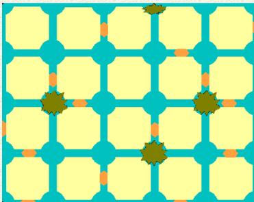
Partially Cemented with Kerogen in Wet Pore System
